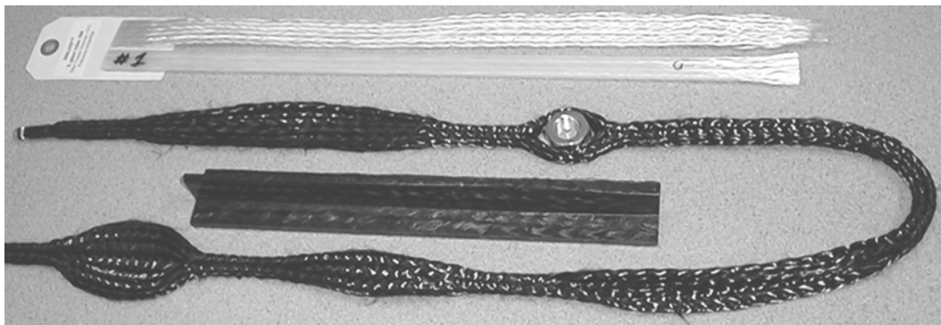
Figure 5. Continuously produced carbon fiber rope illustrating flexibility of 3TEX 3-D braiding process and machine. In the upper part: 3-D braided E-glass strap and pultruded composite.
